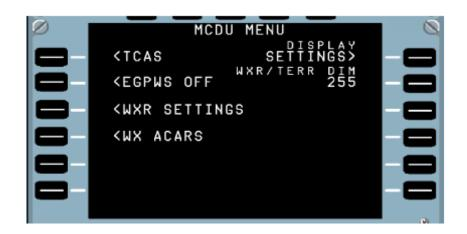
As on the picture above, pushing RSK2 on that page will help you set the WXR/EGPWS image brightness (independently of the actual ND brightness). You can enter here any value from 0 to 255.
